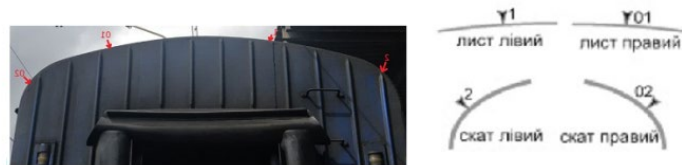
Fig. 3. Scheme of roof sheathing measurements
