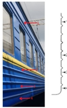
Fig. 5. Scheme of side wall paneling measurements
