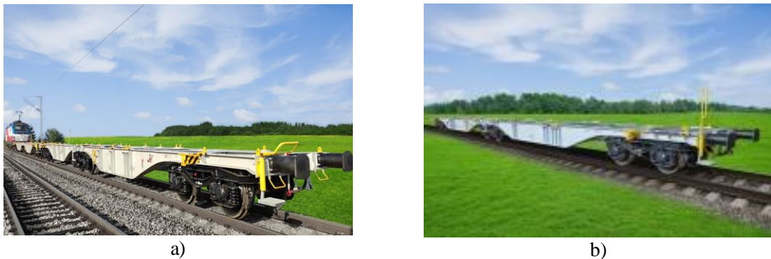
Fig. 6. General view of articulated flat cars type Sggrss 80 (a) and Sggmrss 90' (b) produced by PJSC “KRCBW”
