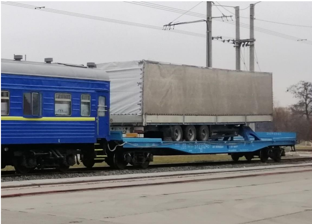
Fig.1. Platform car model 13-9004M with a device installed on it for transporting semi-trailers and loaded semi-trailers
