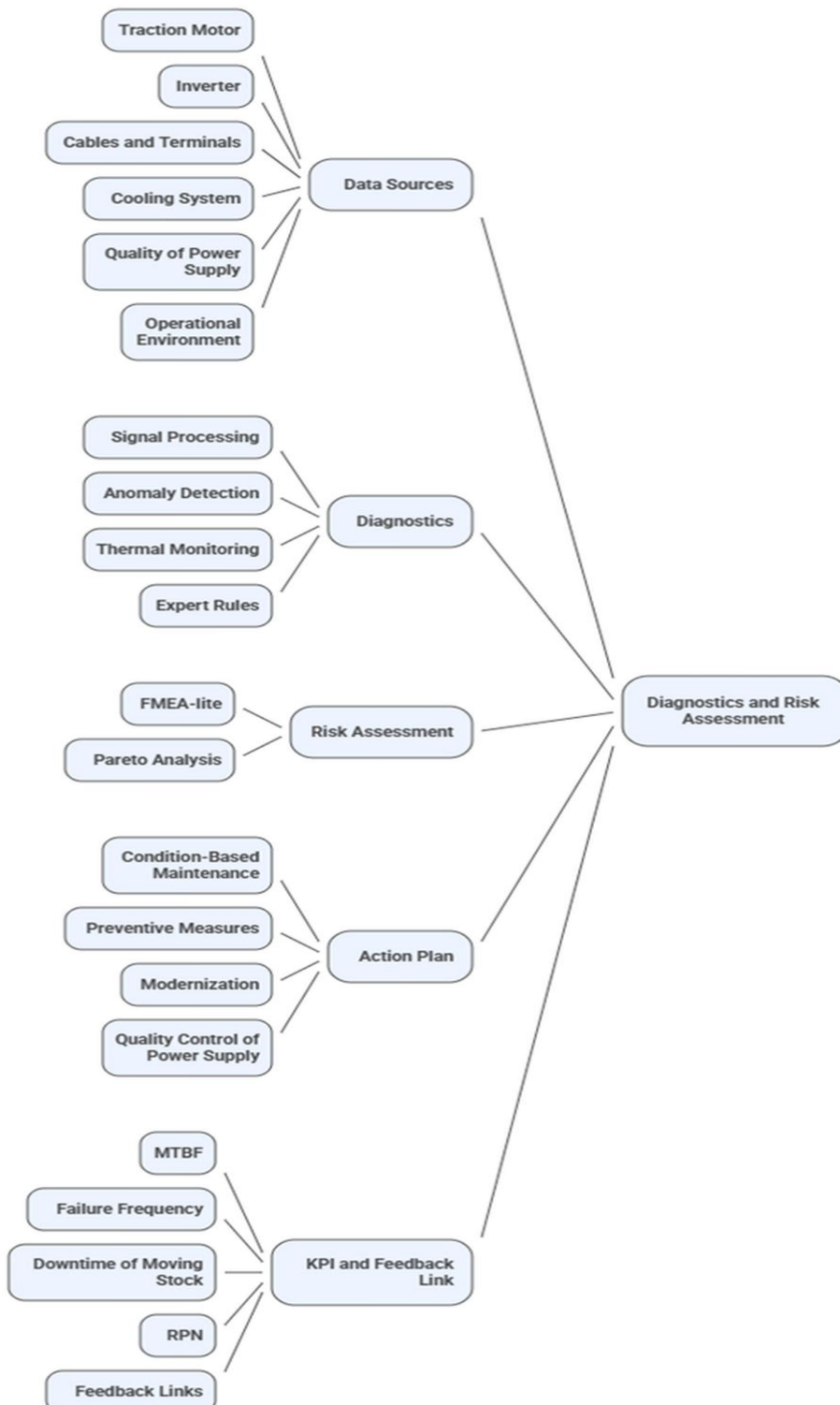
Fig. 1. Conceptual model of integrated reliability management of power equipment in urban electric transport, representing the sequence of stages: data sources → diagnostics → risk assessment (FMEA-lite, Pareto) → Action Plan development → KPI monitoring and feedback.
