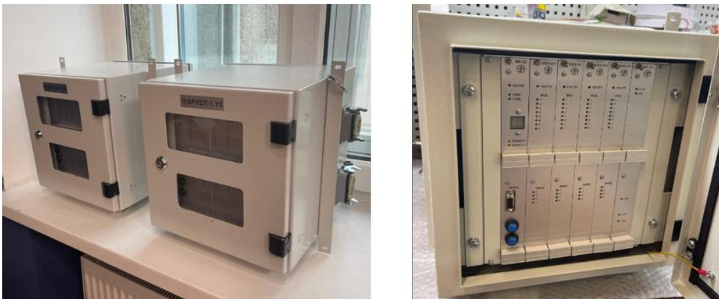
Fig. 5. Practical Implementation of the Intelligent Control System for a Diesel-Generator Unit
